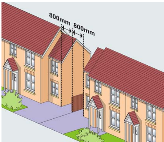
Diagram 9: Good side extension with 800mm retained between the sidewall of an extension and the plot boundary
